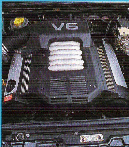
● Audi's 174bhp, 2.8-litre V6 the smoothest here, delivering its power without drama
