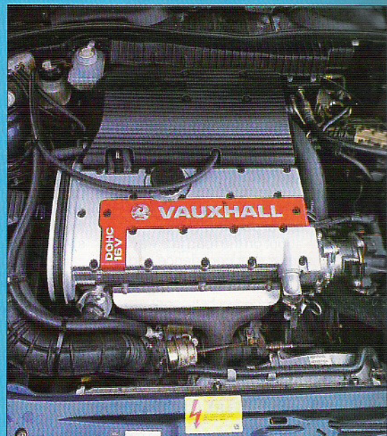
● Vauxhall's 204bhp, 2-litre four prone to high-rev booming, but a fine turbo and a star sprinter
